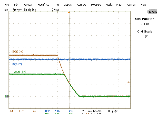
Fig. 27: Simultaneous Tracking a 3.3V input at power-up and shut-down Ch 1 : SEQ(3.3V) Ch 2 :SS(1.8V) Ch 4 : Vout(1.8V)
